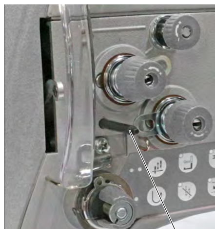
Fig. 12: Locking the machine in place (1)
