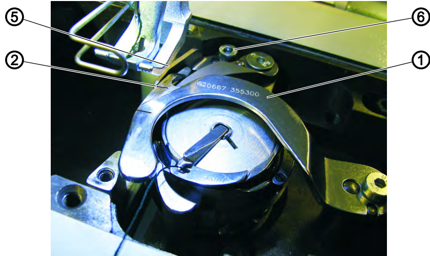
Fig. 70: Setting the cutting pressure
