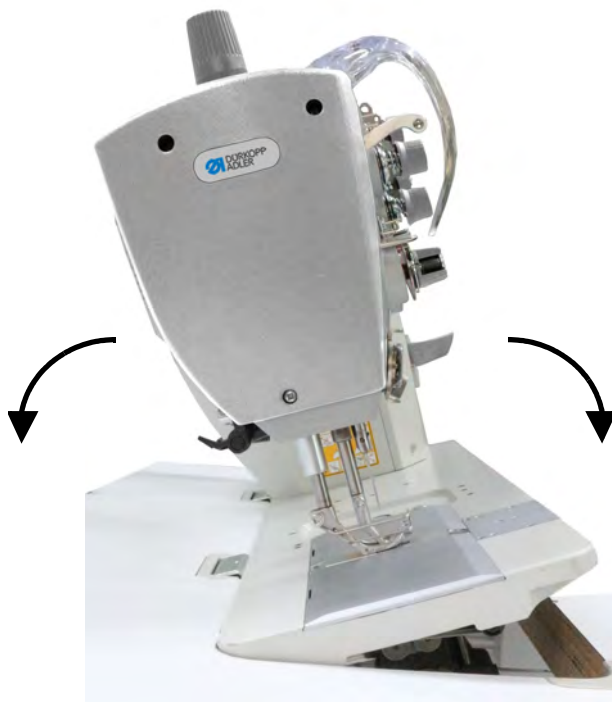
Fig. 1: Access to the underside of the machine
