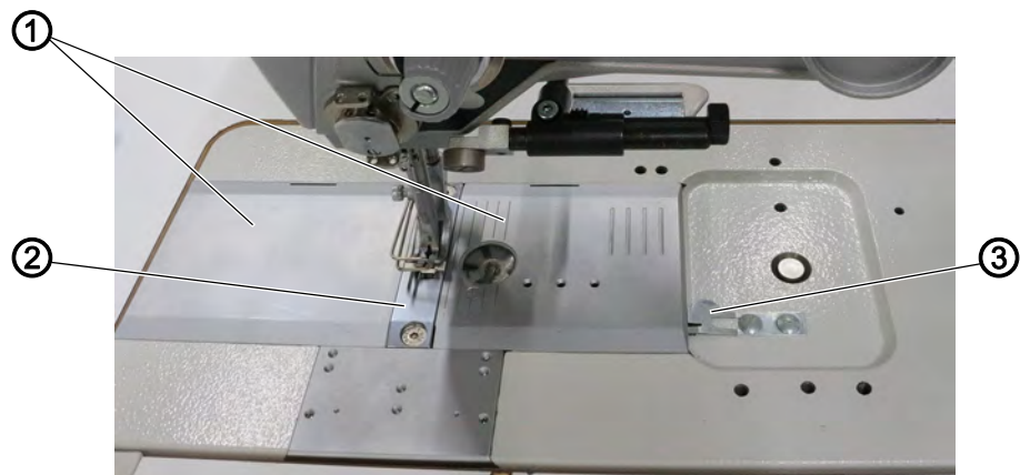
Fig. 8: Opening and closing the throat plate slide
